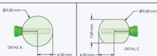
Z2: 9 mm Disc (Width cut at 7 mm)
