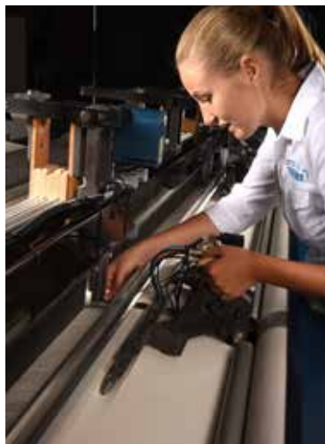
Electronic Leno System (ELSY): drawing in of ends made easy
