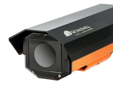
The SMARTIS is TCP/IP Ethernet compliant and therefor analysis and alarm results can be easily applied to PLC. Analog and digital outputs are available for general alarms and direct temperature measurement from specific pixel position or selected area. Due to these built-in capabilities can be used as independent analog output sensor or standalone OK/NOK thermal 2D camera. An image masking system provides you to select only the relevant area/pixel for final evaluation and control.
