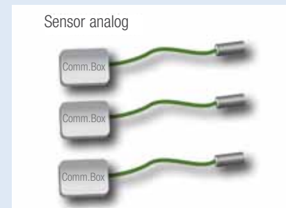
Conventional analog sensors require one box for one sensing head.
