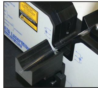
AccuScan 4012 shown with tube sample in V-block
